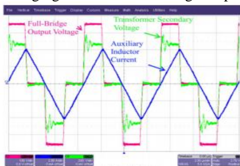
Fig 2: Full Bridge Converter Output
