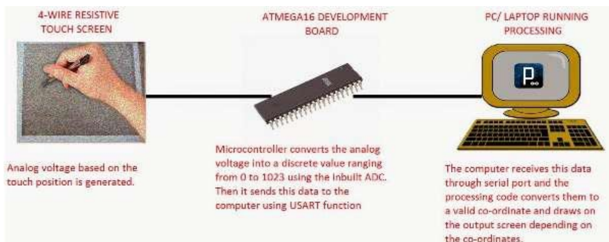
Fig.1. Touch Screen, ATMEGA16 Development Board & PC Running Processing
