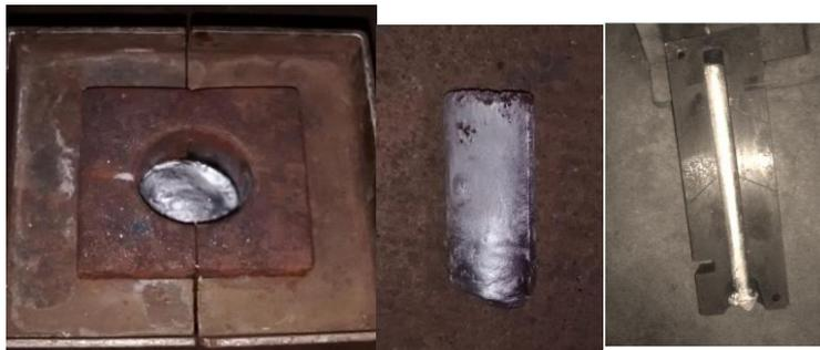
Figure 9::Casting after solidification Cast work piece
