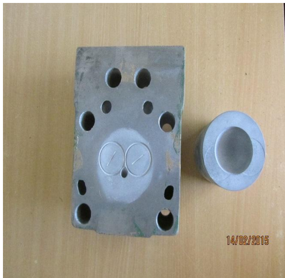
Fig.3 Coated (YSZ material) cylinder head and piston
