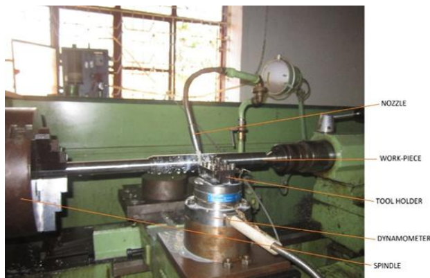
Fig.1: Experimental setup for flood cooling
