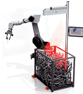
Fig. 3. A graphic of Sick's PLB robotic bin picking system.
