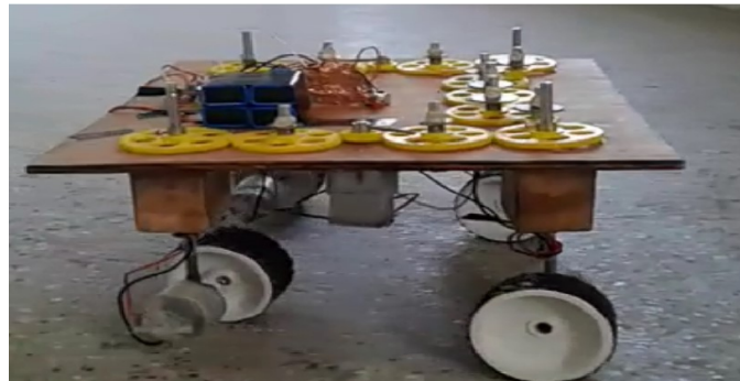
Figure 5: Shafts and Motor installation
