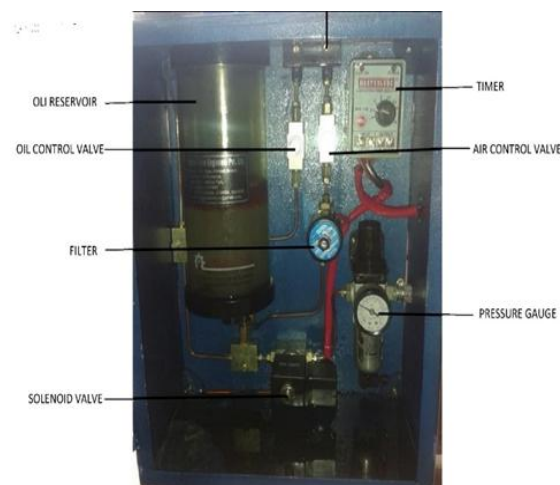
Fig.3: Set-up for Mixing Air and Oil
