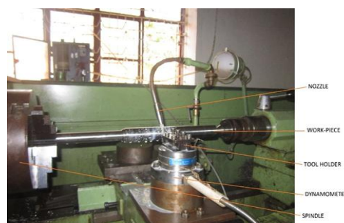
Fig.1: Experimental setup for flood cooling
