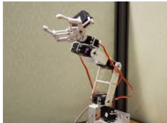
Fig 17 arm for pick and place
