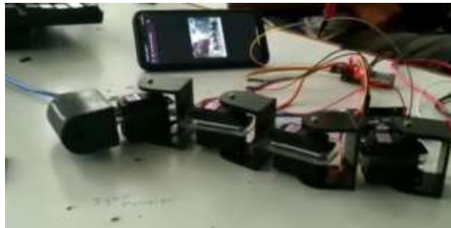
Fig.6: Robotic snake visuals in android mobile connecting through Wi-Fi
