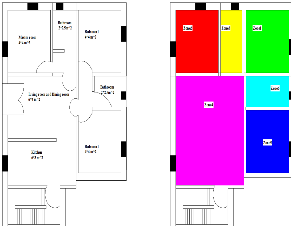
Fig. 4 Floor plan of the building: north (equator) at the right of the plan (a) House plan, (b) House zones
