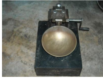
Fig 4 Casagrande's liquid limit apparatus
