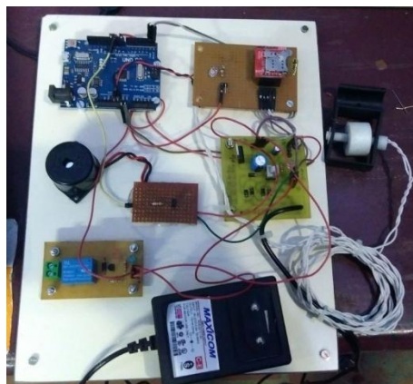
Figure (3) Reed Switch interfaced with Arduino and GSM Module
