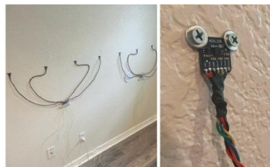
Fig. 36: Experimental Setup for Modeling Vibration Dissipation
