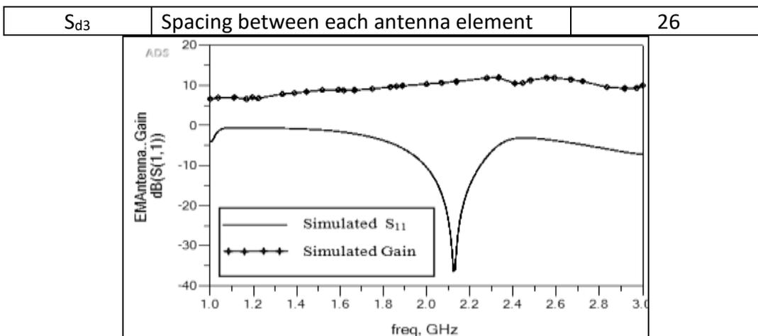
**Figure 2 Simulated S<sub>11</sub> and Gain of the Single Element Yagi Antenna**
