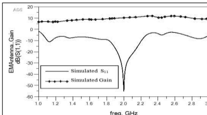
**Figure 4 Simulated S<sub>11</sub> and Gain of the 1x4 Yagi Array Antenna**
