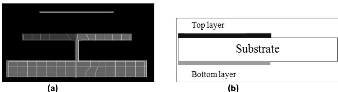
**Figure 1 Single Element Yagi Antenna (a) Top View (b) Side View**
