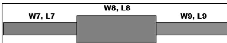
Figure 7 Stepped Impedance Low Pass Filter
