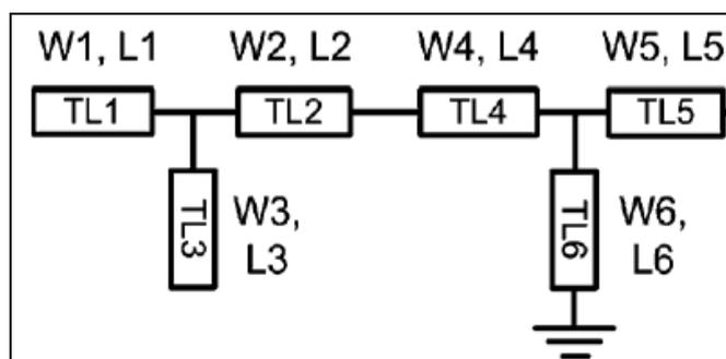
Figure 6 Topology of the Matching Circuit
