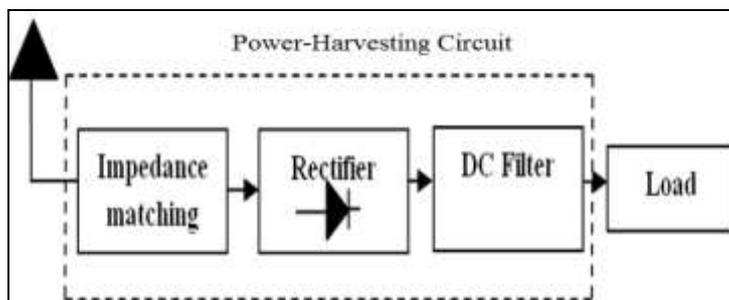
Figure 5 Block Diagram of Rectenna
