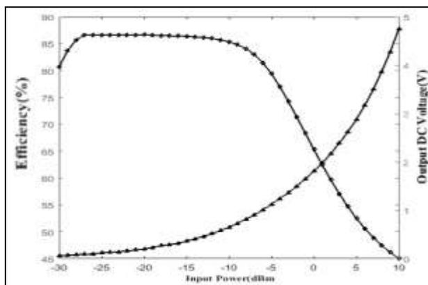
**Figure 9 Simulated Efficiency and Output DC Voltage of the Rectifier for Different Input Power Levels**
