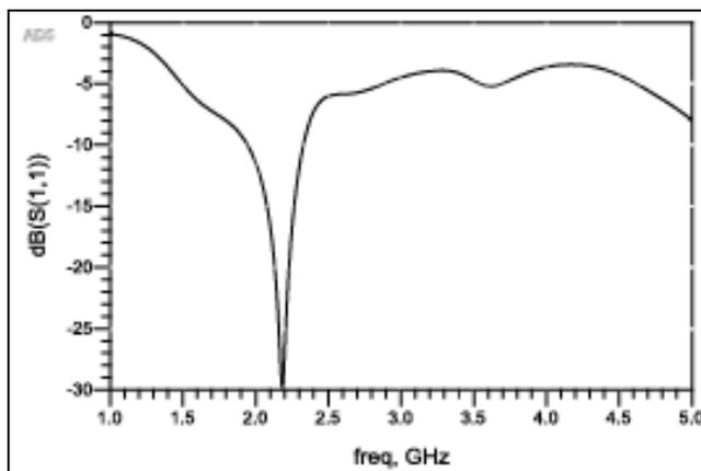
**Figure 8 Simulated Return Loss of the Rectifier**
