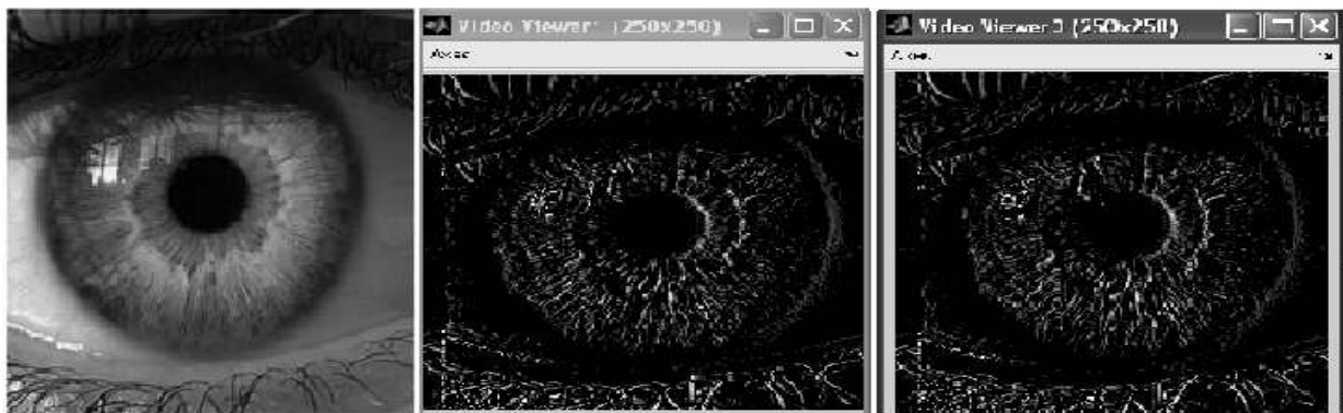
Figure 8a) Original image b) Simulink software output c) Emulator FPGA output
