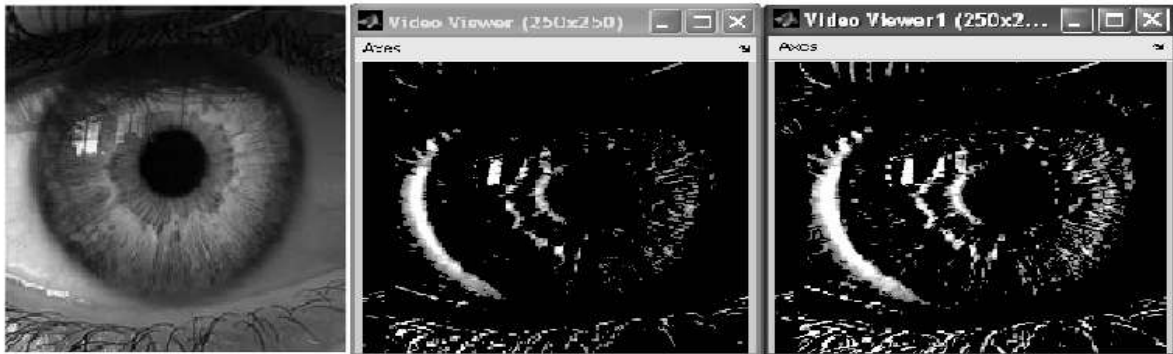
Figure 7 a) Original image b) Simulink software output c) Emulator FPGA output
