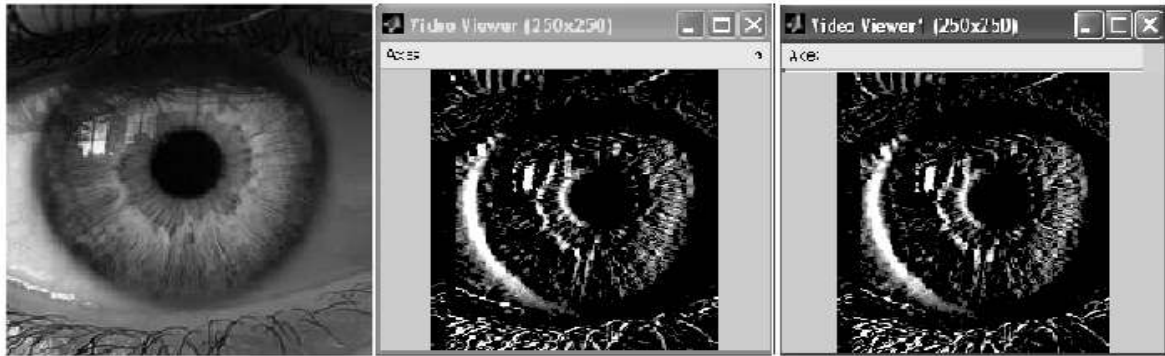
Figure 6a) Original image b) Simulink software output c) Emulator FPGA output
