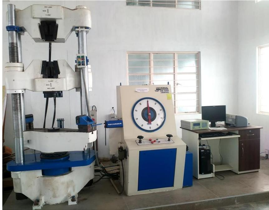
Fig.2 Computerized - Servo controlled Universal Testing Machine
