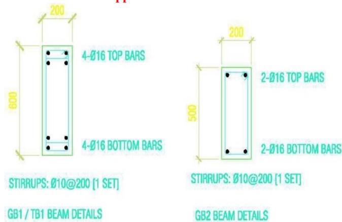
Fig 4.2 Plinth Beams
