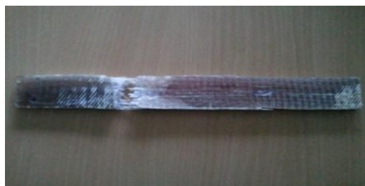
Fig 2.4 Laminate after Applying Tensile Strength
