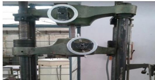
Fig 2.3 Composite Laminate on Universal Testing Machine
