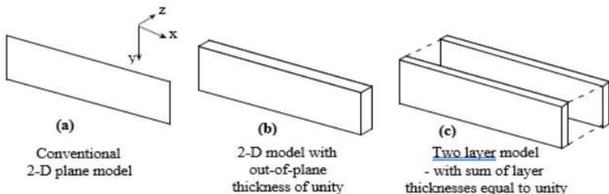
Figure 2 Finite element modelling techniques: (a) conventional plane model with no out-of-plane thickness, (b) one layer model with out-of-plane thickness, (c) two layer model with layers of different thicknesses
