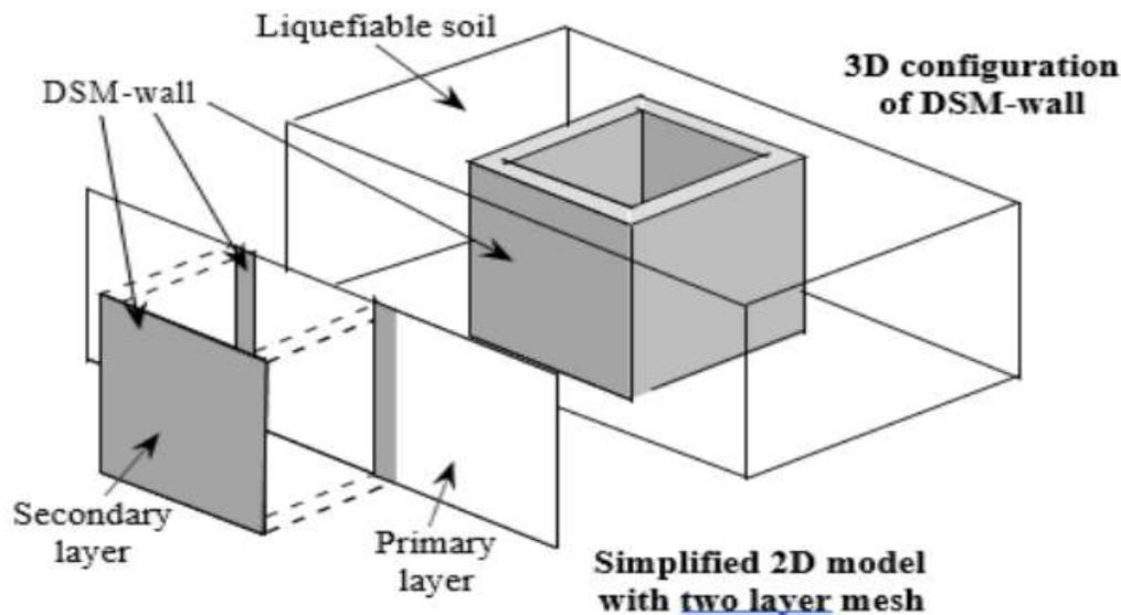
Figure 3. Simplified 2-D modelling of the 3-D configuration of a DSM-wall using a two layer mesh
