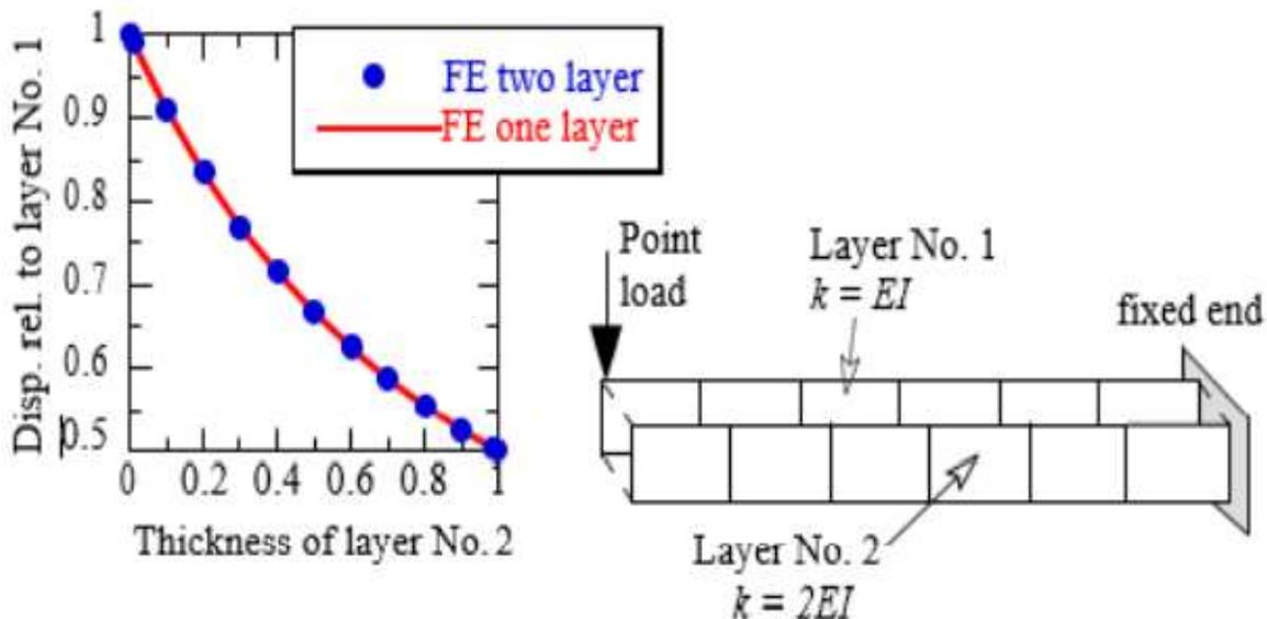
Figure 4 Comparison of theoretical and two layer cantilever beam results
