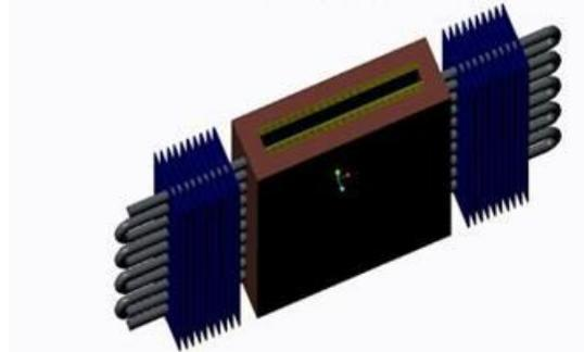
**Figure 3: Bend type Heat Pipes**
