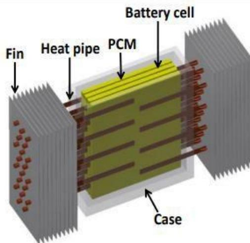
Figure 1: 3D model of Battery pack setup
