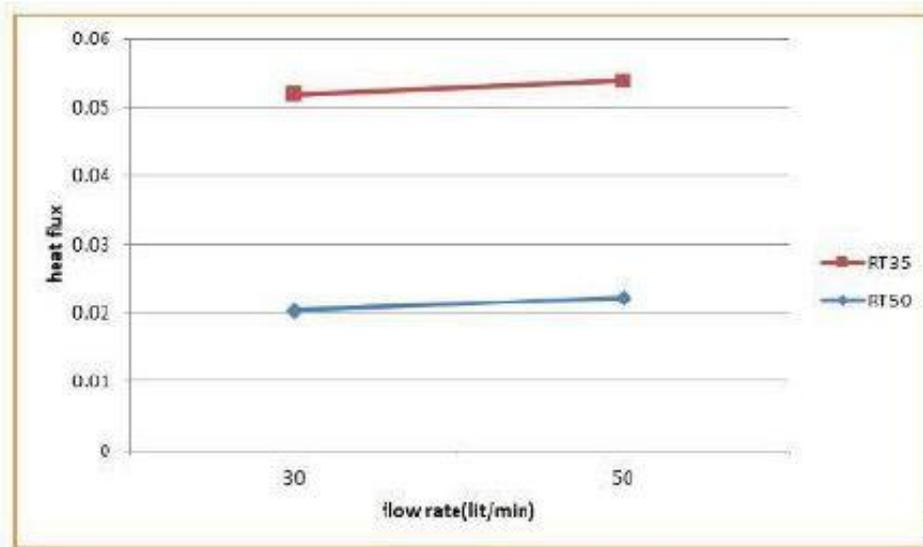
According to the plot, the maximum Heat Flux is Possible with RT 35 over RT 50
